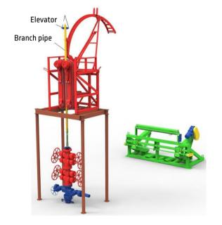
5. To descent upper terminal element lower the injector and fix it on the elevator.
