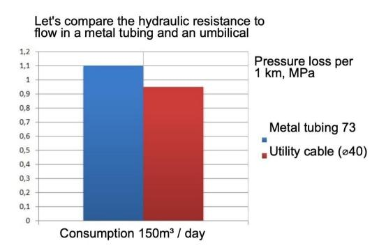
As a result, hydraulic fluid resistance in umbilical with inner diameter 40mm is in practice equal to the resistance of tubing string NKT 73.
