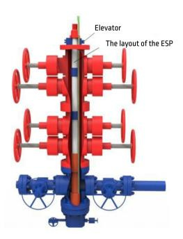
3. Install injector, lifting equipment. Install the reel with umbilical into launching equipment and to put the umbilical into injector. Connect umbilical with components of ESP and splice conductors of umbilical. Descent the unit.
