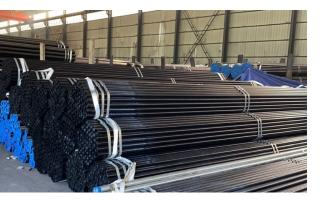
Seamless Steel pipes from 1/4" to 20" in schedules 10s, 40s, 80s, 160 and XXH. Standards A213, A268, A269, A789 in grades
